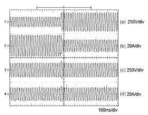
Fig14: Experimental results of the proposed AVR upon changing the utility voltage abruptly from 77 to 143 V. (a) Utility voltage. (b) Utility current. (c) Load voltage. (d) Load current.
