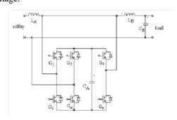
Fig 2: Circuit configuration of the proposed threearm AVR.
