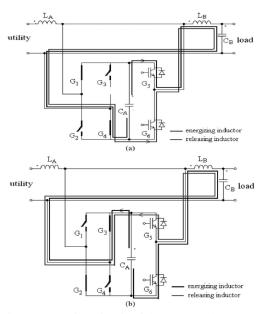
Fig. 5. Operating circuit of the proposed AVR under the ac buck mode (a) Positive half-cycle. (b) Negative half-cycle.
