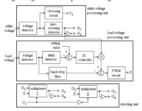
Fig. 7. Control block of the proposed three-arm power converter.
