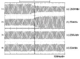
Fig13: Experimental results of the proposed AVR upon changing the utility voltage abruptly from 143 to 77 V. (a) Utility voltage. (b) Utility current. (c) Load voltage. (d) Load current.
