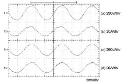
Fig.8. Experimental results of the proposed AVR under a utility voltage of 143 V and resistive load. (a) Utility voltage (b) Utilitycurrent (c) Load voltage (d) Load current.
