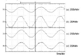
Fig.10. Experimental results of the proposed AVR under a utility voltage of 77 V and resistive load. (a) Utility voltage. (b) Utility current. (c) Load voltage. (d) Load current.
