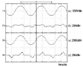
Fig. 11. Experimental results of the proposed AVR under a utility voltage of 121 V and nonlinear load.
