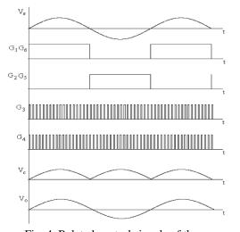
Fig. 4. Related control signals of the power
