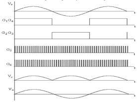
Fig. 6. Related control signals of the power electronic switches and voltage waveforms of the proposed AVR under the ac buck mode.
