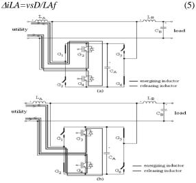
Fig. 3. Operating circuit of the proposed AVR under the ac boost mode. (a) Positive half-cycle. (b)
