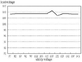
Fig12: Experimental results of the load voltage for the proposed AVR upon varying the utility voltage from 77 to 143 V.
